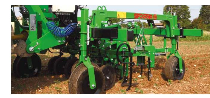
> Bio Theser is a machine for inter-row and inter-plant weeding of organic crops, where the use of chemicals is not allowed. Easy to adjust, precise in work and reliable
