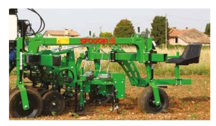
**Bio Thaves** is equipped with an electro-hydraulic guide system to ensure maximum precision in alignment between elements and crops. The elements are assembled on a mobile frame that guarantees a maximum excursion of 25 cm. The movement of the elements along the rows is managed by an operator using a joystick and sitting at the rear of the implement.
